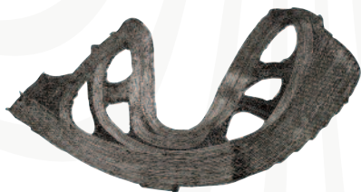
High Volume - Tailored Fiber Placement (HV-TFP)
